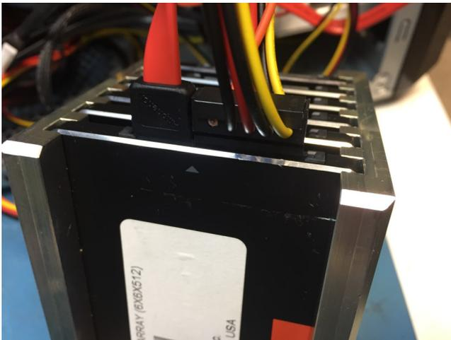
Turn on the backup station and let the software run. You should see the SSD display in the main window (see next page) by itself. If it does, turn off the system, and connect the cables to the next drive and continue the process until all drives have been tested.
