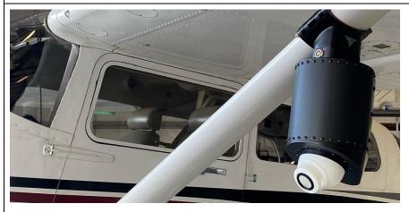
Wing mounting allows the user to transform a regular airplane into an efficient inexpensive aerial survey airplane. The installation can be done in a couple hours by an airframe and powerplant mechanic without making any permanent modifications to the airplane. The Meeker wing strut attachment shown here is FAA STC certified for the Cessna 172, 182 and 206.
